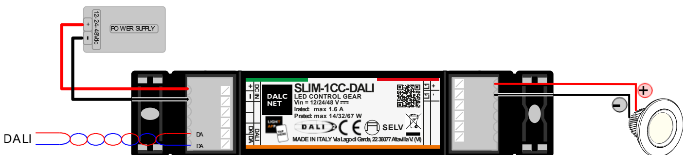
Figure 2: Connection diagram for White or Single-Colour LED loads
